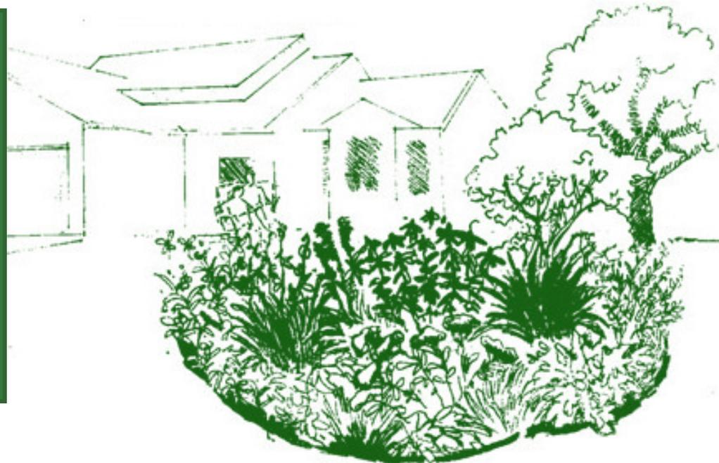
*Rain gardens are constructed by digging a shallow depression in a well-drained area, and planting with a variety of flood-tolerant plants.*
